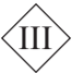
Class III product: Designed to be supplied from a separated extra low voltage supply (SELV). The voltage from a SELV supply is low enough that a person can normally come into contact with it without the risk of electric shock.
